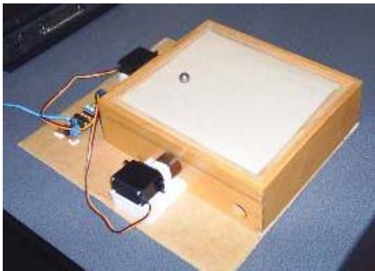
Fig. 2. The controlled object „plate and ball”
